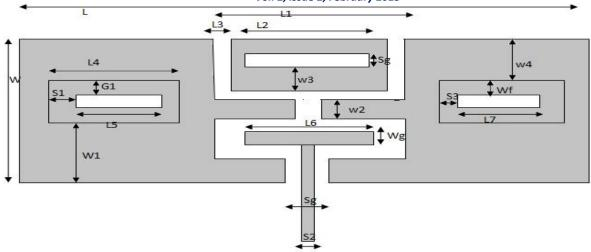
Fig.1 Antenna confiuration structure Of The Low Profile Printed Monopole Antenna For RFID Applications
